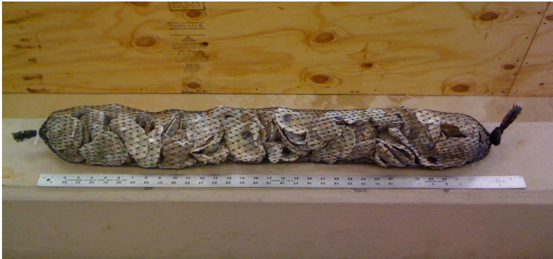
Figure 3: Photo of a completed oyster shell bag that is used in testing. The bags are nominally 0.076 m (3 in) in diameter and 0.82 m (30 in) long. A total of 120 bags are produced for the testing.
