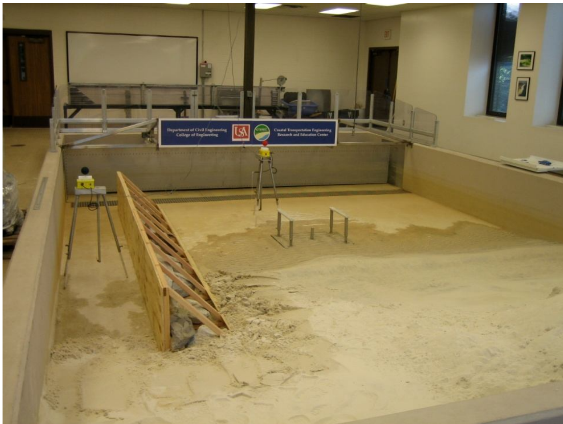
Figure 2: Photo of the basin at the University of South Alabama after installing the splitter wall and re-sloping the beach face.
