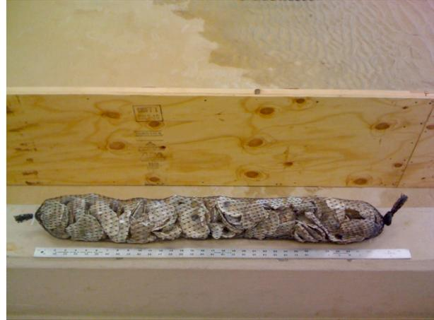
**Figure 2:** Completed oyster shell bag before testing.
