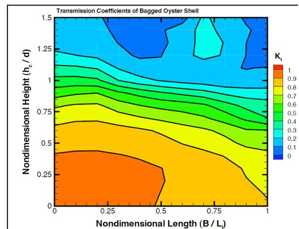
**Figure 4:** Non-dimensional relationships of the structure and the incident wave height to the wave transmission coefficient.
