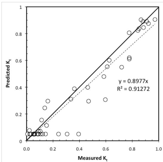
**Figure 3:** A comparison of measured and predicted transmission coefficients using the predictive equations of Van der Meer et al. (2005). Open symbols (o) represent measured data, the dashed line is a linear regression with a zero intercept, and the dark solid line represents perfect agreement.
